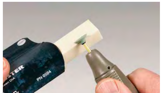
The SHOFU Adjuster, made of alumina, is ideal for instrument cleaning and individual shape adjustment (see page 50).
